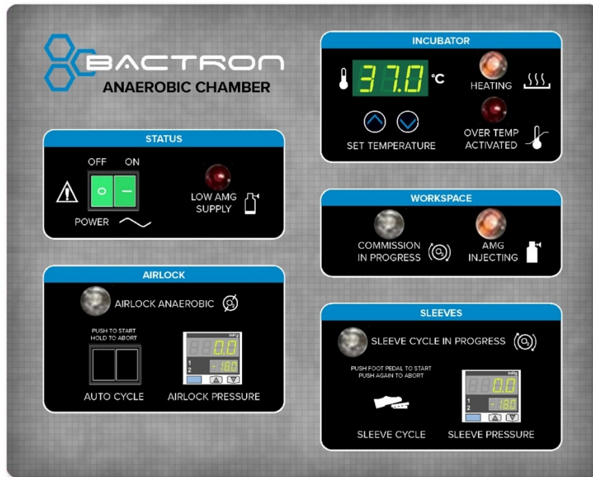
Figure 5: Main Control Panel
